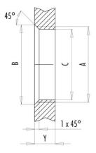
Installation direction: o-ring sits on chamfer.
